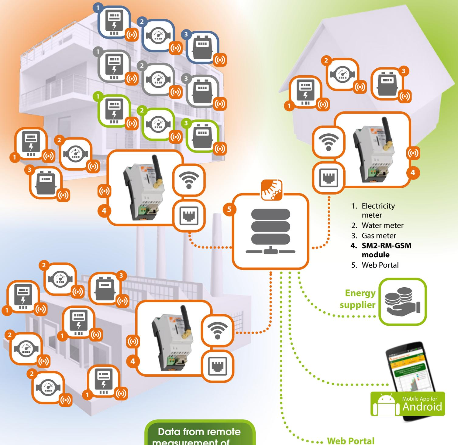
**Data from remote measurement of devices with S0 output such as:**
